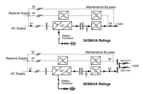
Figure 4 – Utility Supply failure
